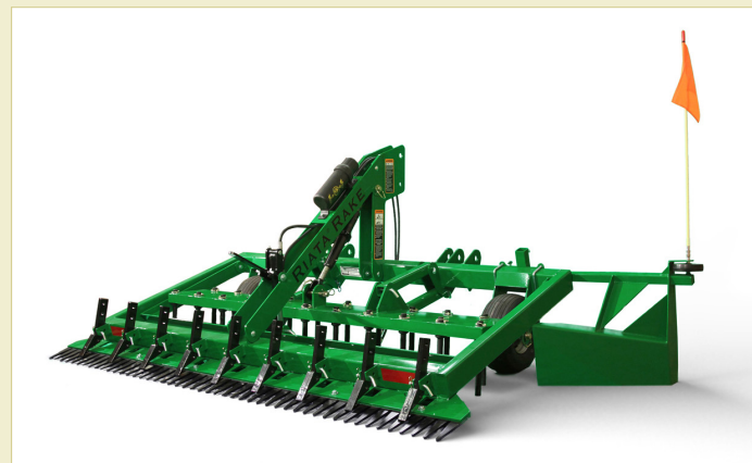
Both the 1108 and 1110 models are compatible with tractors that support a Category 1 or 2 three-point hitch. (iMatch and Quick-Coupler compatible.)
