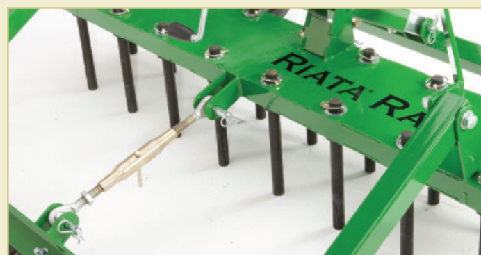
Both the 1108 and 1110 models are compatible with tractors that support a Category 1 or 2 three-point hitch. (iMatch and Quick-Coupler compatible.)
