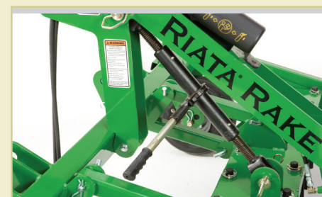
Control your working depth by rotating the ratchet jack to raise or lower the tines. Ratchet jack works independently of the rear finishing comb.
