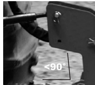
Incorrect - lengthen the top link
